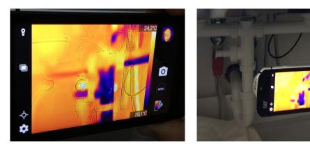
Figure 1.10: Thermographic equipment to measure temperature differences
