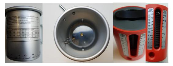
Figure 1.9: Flowmeter equipment to measure the flow at fixtures
