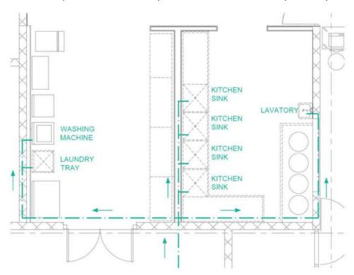
Figure 1.6: Example of a domestic water distribution system for a commercial kitchen
