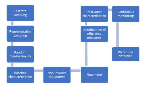
Figure 2.2: Example of a sampling approach
