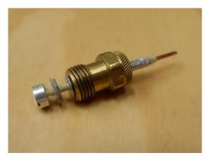
Figure 1.6: Thermocouple connection for pipes
