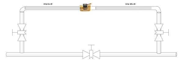
Figure 1.12: Mechanical water flow equipment (invasive)
