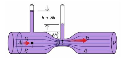
Figure 1.2: Working principle of venturi flowmeter
