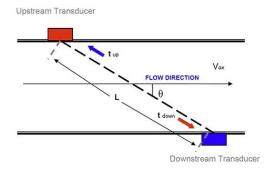
water from outside of the pipe by shooting pulses of sound through the pipe walls, thus having application flexibility and making them suitable for water flow measurements in large pipes.
