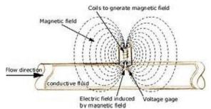
Induction, according to which liquid generates voltage when it flows through a magnetic field. The more rapid the fluid flow, the more the voltage generated. The voltage produced is directly proportional to the water movement; the voltage signal is processed into the volumetric flow rate by the electronics. Since the magnetic flow meters show an intermediate accuracy, they are not
